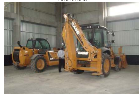
Telehandler and Back Hoe Loader
